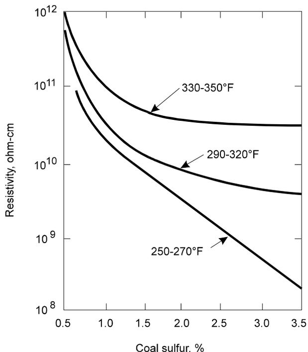
Figure 3-3. Fly ash resistivity versus coal sulfur content for several flue gas temperature bands
