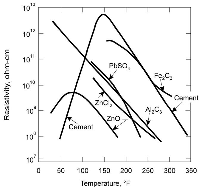
Figure 3-1. Resistivity of six different dusts at various temperatures
