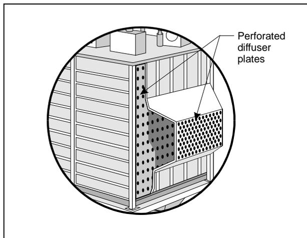
Figure 3-7. Gas inlet with perforated diffuser plates
