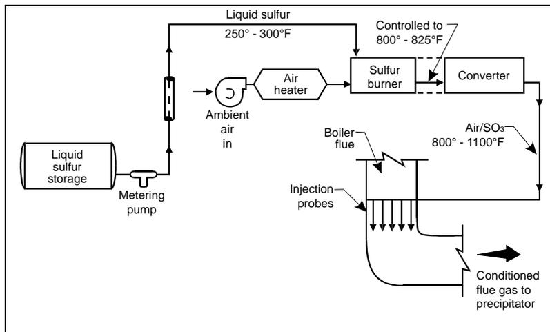
Figure 3-4. Flow diagram of sulfur-burning flue gas conditioning system
